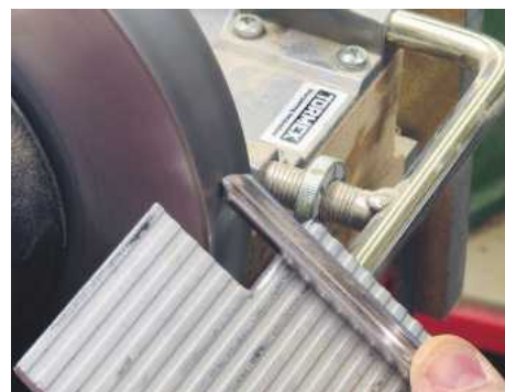
▲ Pic.2 This is probably one of the simplest tools to sharpen. Set the platform to the right angle and gently rotate the tool to sharpen it. To prevent putting a point on it, rotate the tool slowly as the flute becomes more upright
